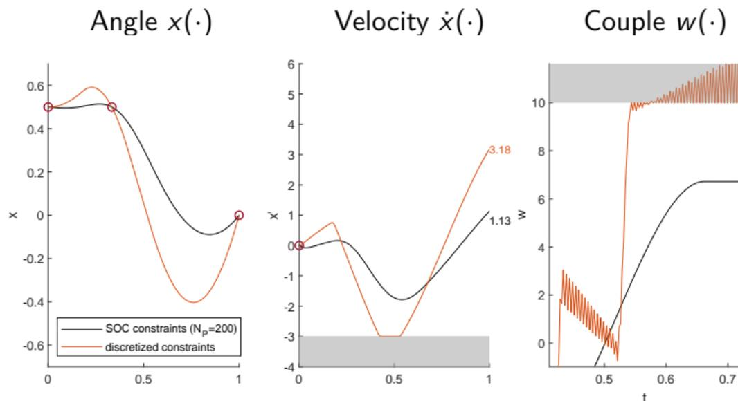
**Figure:** Comparison of SOC constraints (guaranteed  $\eta_w$ ) vs discretized constraints ( $\eta_w = 0$ ) for  $N_p = 200$  - Chattering phenomenon like for traffic cameras!.
